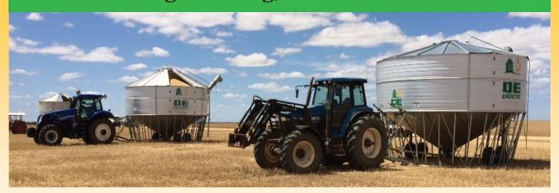
Stronger: DE field bins are engineered with the heaviest wall section and base construction in the industry, guaranteeing they won't crumple during loading. We equip these bins with heavy-duty 2-tonne axles, 'New' Landcruiser tyres and rims for superior durability. Larger bins come standard with walking beam axles, and all bins are fitted with PTO slip clutches to protect the driveline.
