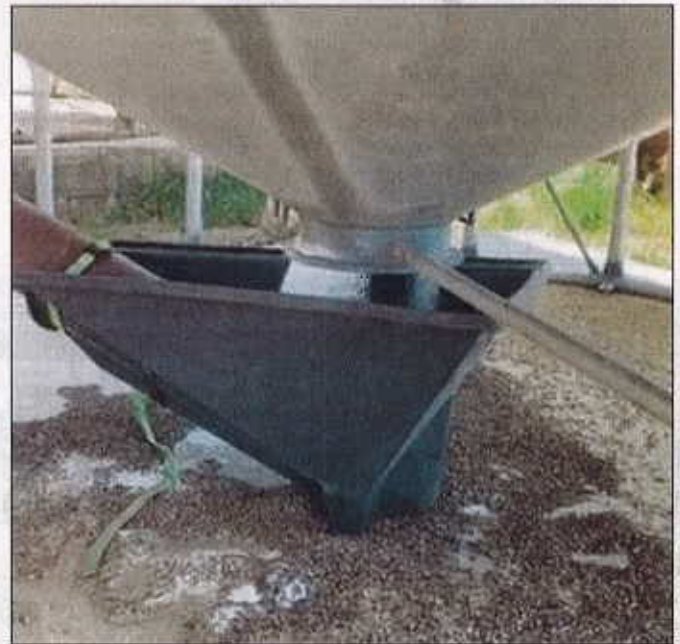
□ DE Engineers' standard cone design works well in its new fertiliser mobile field bin. "You don't need a steeper-angled cone for fertiliser," company principal Kevin Prater said.
